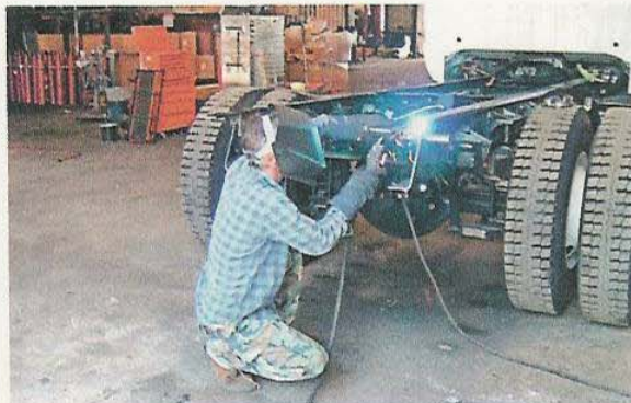
Double A Body Builders has 23 MIG welders, all of which use argon/CO2 shielding gas mixture to minimize spatter spatter. The MIG wire feeders are located about 30' from the shielding gas piping system.
