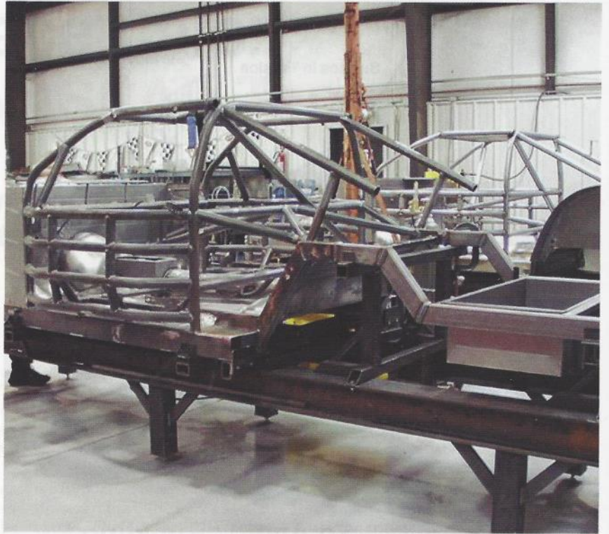
Fig. 5 — The material of this frame is specified as mild steel. NASCAR dictates the safety cage design, tubing size, and wall thickness.
