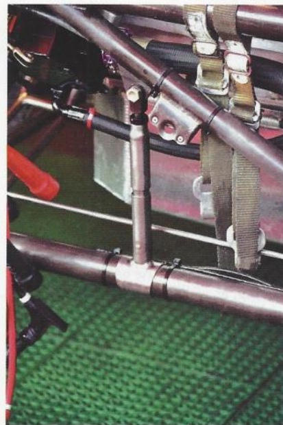
Fig. 4 — This unique frame support was observed in a dragster chassis using heat-treated 4130. It appears to be designed to limit movement of the frame components to prevent local buckling. A dragster does not use springs; the chassis flexing provides the needed suspension.
