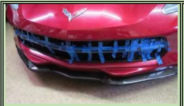
Did the same for the 2<sup>nd</sup> side with another batch of epoxy. The butted center fit perfectly. This time I put a somewhat larger amount on the wider part of the Overlay where it had felt slightly loose until I held it in place. As with the first side I put additional strips of tape along that whole section. It felt very secure, no need to hold it in place.
