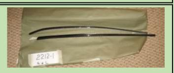
The two Overlays are the exact same shape as the two piece chrome bar. They are shaped the same, where the chrome is wide and rounded at the ends, so are the CF parts. Where it narrows to  $\frac{1}{2}$  inch in the center- so does the carbon fiber Overlay. Each is ~25 inches long
