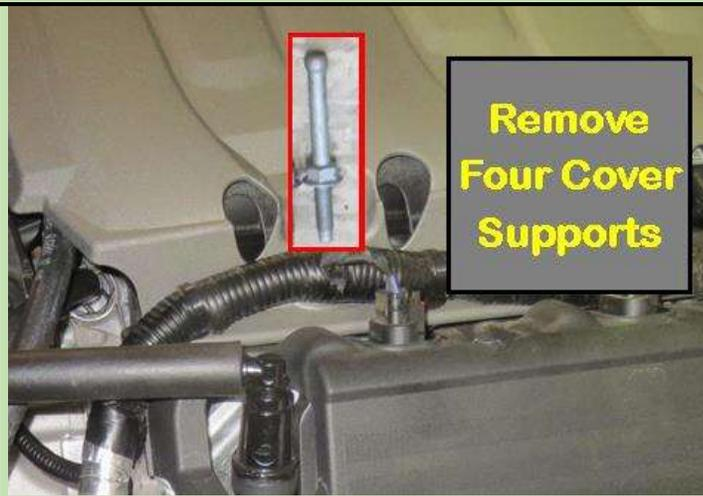
After removing the valve cover- plastic covers there are four long studs that need to be removed. These have a 10mm nut at the bottom. Thought this would be easy as I just needed to use my 10mm deep socket. However, the balls on the stud top were larger than the socket ID near the top! Was able to wedge a 10mm box end wrench on the nuts. Fortunately, it only required a slight turn to loosen since that is all the room available! They then unscrewed by hand.
