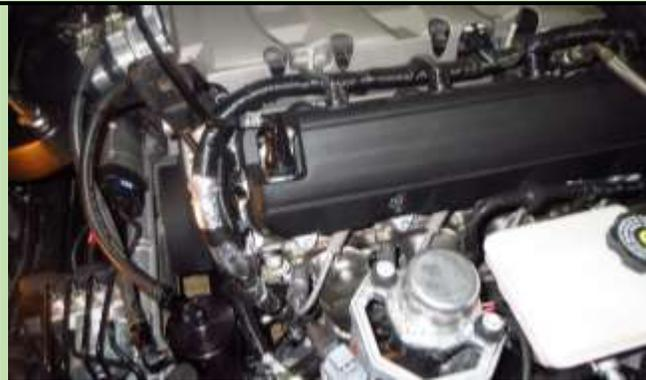
Removed the driver's side plastic rocker arm cover. Comes off with your fingers. See 2014 install that follows for details.
