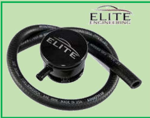
from the oil tank is passed through media in the “oil separator” that replaces the oil inlet cap. As shown in the above picture, this cap replacement is higher and if disassembled contains similar media as the “catch can.” The air and oil mist enter the bottom of the can and the mist can agglomerate into oil droplets that fall back into the tank. It has to be removed when adding oil, at which point it can also be disassembled by unscrewing the outer shell and the parts cleaned.
