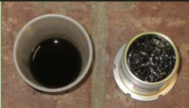
This is a top view. As with all the construction, the threads are cut perfectly and screw precisely into the inside machined top of the can. Very professional. Had there been more accumulation, would have run mineral spirits through the stainless ribbon to clean it.
