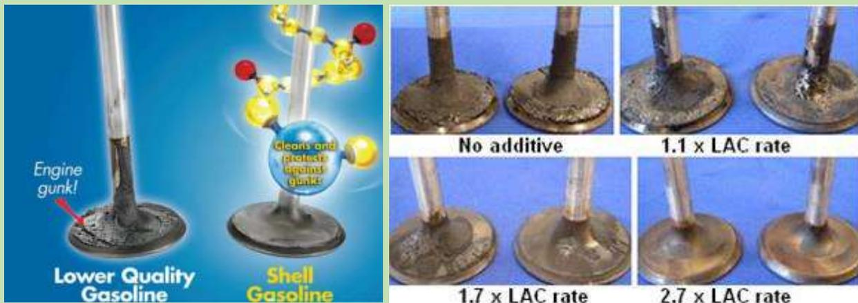
The picture left is from Shell and shows “coking” without their cleaning additive and a clean valve with it. The picture right shows “coking” without cleaning additives and with varying amounts added; 1.1, 1.7 and 2.7 units. As noted, it gets less with added amounts.
