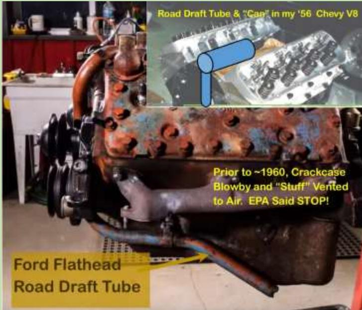
Recall the one on my '56 small block V8 Chevy. It consisted of a soup can size container filled with steel wool that was located in the lifter valley under the intake manifold. It had a ~3/4 inch diameter tube attached that went from the can and exited near the bottom of the oil pan. When the car was moving all the blowby and other “stuff” in the crankcase came out in the atmosphere. If you burned oil, “smoke” would come out from under the car. Not good for the environment! In the 1960’s the EPA
