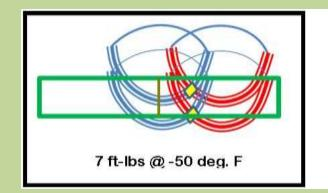
The above schematic shows the lowest toughness specimen produced. It had about 50% single refined material but that was placed in the center of the Charpy specimen or as Dr. Nelson would say most of the refinement was wasted! It matched the 8 ft-lbs in the prior process variations tests!
