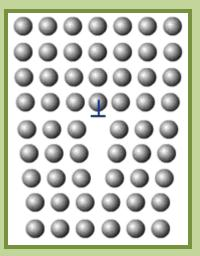
**Dislocations** are usually arranged in what are called edge and and screw type а combination of these structures. Sufficient to sav for this discussion; as the material is strained the crystal structure on one side of the dislocation may form a strong bond with those atoms on the other side of the void.
