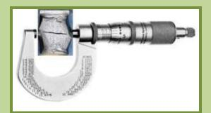
The deformation of the outer edges can be measured with a micrometer. Of interest the amount of deformation beyond the original 10 mm (0.394 inches) when measured in thousands (Mils) is often about equal to the energy absorbed in ft-lbs! Some specifications ask to have this Mils Lateral Expansion and well as the % Shear, as observed in the broken face, recorded.
