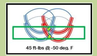
The above schematic shows the toughest Charpy in the series. It had double refined material (yellow area) at both outer edges of the specimen. It
