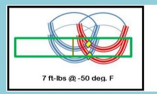
The above schematic shows the lowest toughness specimen produced. It had about 50% single refined material but that was placed in the center of the Charpy specimen or as Dr. Nelson would say most of the refinement was wasted! It matched the 8 ft-lbs in the prior process variations tests!
