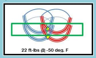
The toughness was somewhat higher at 22 ft-lbs. In general it does say that in this Mn Mo weld metal the doubly refined material is tougher that single refined material. It clearly shows that when the refined material is placed at the outer edges the toughness is significantly higher.
