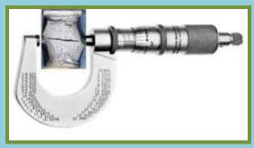
The deformation of the outer edges can be measured with a micrometer. Of interest the amount of deformation beyond the original 10 mm (0.394 inches) when measured in thousands (Mils) is often about equal to the energy absorbed in ft-lbs! Some specifications ask to have this Mils Lateral Expansion and well as the % Shear, as observed in the broken face, recorded.
