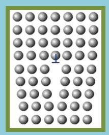
Dislocations are usually arranged in what are called edge and screw type and a combination of these structures. Sufficient to say for this discussion; as the material is
