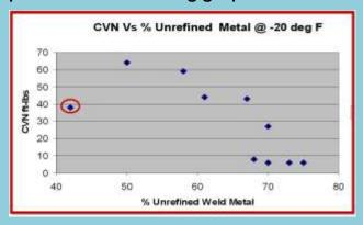
Again there is good correlation with the toughness and percent unrefined weld metal. Therefore the reheated area (HAZ) of the previous weld bead has a more refined metallurgical structure and higher toughness. There is one anomaly that as above will be explained in subsequent tests.
