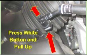
Next remove the line that brings filtered air into the crankcase so it can come out with the PCV purge system. There are a number of these hose clamps used on the C7. There is a white tab that can be seen in this view. Press in and pull up the hose connector. This plastic tab springs back so it grabs onto a hose barb.
