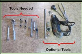
You'll need a 3/8 ratchet wrench, 7 mm, 10 mm and 7/16 inch sockets. A 7 mm and 10 mm deep socket are also useful. Several extensions and a 10 mm open end wrench are also a help. A small Phillips screw driver is needed to remove the OEM MAF.
