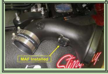
Installed the Mass Air Flow sensor into the new duct. Where GM used sheet metal screws in plastic, aFe uses molded in metal threaded inserts and they provide the matching screws. Very well done.
