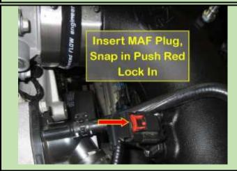
Next step is to install the MAF plug. Simple to do if you did not remove the red blocking clip, as I did! Just push the plug into the MAF socket you installed and then push-in the red blocking clip. The red clip just prevents access to the black tab below that secures the plug in the socket.
