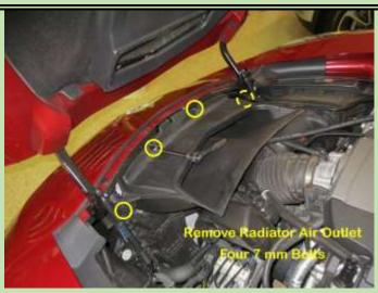
First thing to remove is the duct that takes air from 1/3 of the radiator and ducts it out the hood vent. This is straight forward, you'll need a 7 mm socket and a ratchet. You can use a long extension to remove the two center bolts and the one on the driver's side. But a short one or hand ratchet is needed for the passenger side. There is a bolt in the center but it is not holding the air duct, so don't remove.
