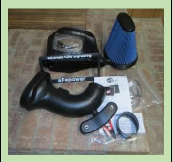
This is what is in the box. Everything is very well made and rugged. The oiled filter comes in a separate box with instructions on how to clean and re-oil. Note, a low restriction non oiled filter is also available. It doesn't have as high an airflow as the oiled cotton but some folks don't want to deal with the mess of cleaning and very carefully oiling the filter.
