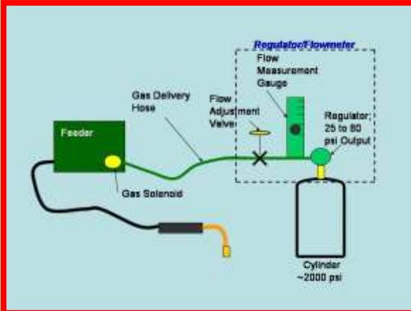
To keep flow at the preset level the gas pressure in the cylinder regulator will be between 25 and 80 psi. Flowgauge regulators (those with a flow calibrated pressure gauge) operate in this pressure range as well.) However to flow shielding gas though the welder and torch typically requires 3 to 5 psi depending on restrictions.
