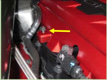
Install the left rear bolt first by hand and only about halfway. That is an easy one to access and positions the cover properly so the other 3 holes will be aligned.
