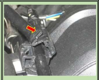
Place the hose in front of the engine cover out of the way. Best to keep the clip attached and remove it after. One of these "Professional Youtuber" videos showed removing it while the cover was attached. Bad idea! They took quite a while and needed several tools. In the end the hacked-up the plastic barbs that holds the clip in place and showed it was very loose when they reinstalled.
