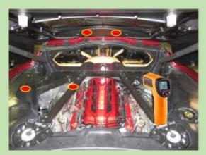
Had several adhesive double-sided tapes including a Gorilla brand outdoor tape that was good for 225 degrees. Decided to check what the engine compartment temps after driving for >1/2 hour with the engine water temp at 185 F and engine oil 175 F. Temps in the areas shown with red circles were all between 100 to 105 F. Particularly where the lights would go it was 100 F. Might heat soak
