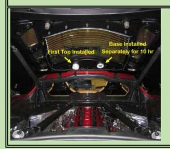
This pic, shows the base on the right that was attached to the hatch after cleaning with a grease, wax and oil remover solvent. Placed both halves, which are very light, on the hatch for ~10 hours so they adhered with minimum holding requirement.
