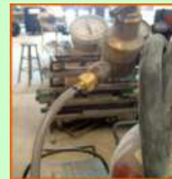
their standard ¼-inch ID gas delivery hose, the peak flow rate was over 150 CFH at each weld start. Any flow rate over 40 CFH, with their 3/8 inch ID MIG gun nozzle, creates turbulence, pulling air into the gas stream, creating excess spatter. With the **GSS**, peak surge was about 45 CFH for only a short time, but it is enough to quickly purge air from the weld start area.
