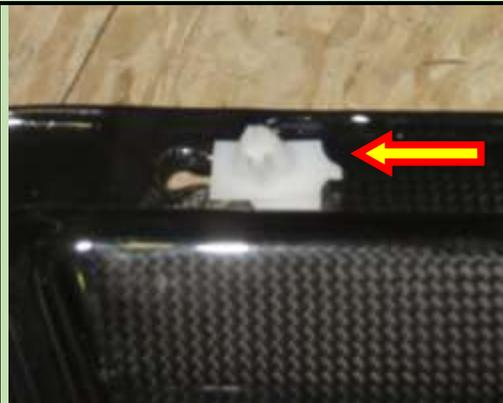
Note, there are thin rubber type washers that fit over the clips. They are probably used to stop rattles. They just slip over the clip tip.
