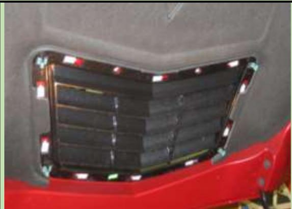
This was my “one person” solution! On one corner I placed a rag around one of the vents. Then pulled with my right hand while pushing from the front of the hood on the edge of the vent with my left. It took quite a bit of force, however when it released, all but the opposite side two clips popped loose!
