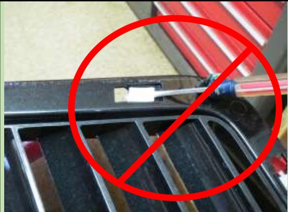
Here is the clip being reinstalled in the CF Hood Vent. Be sure they are all in the correct location and facing the proper direction. Insert from the top side with the clip facing up.
