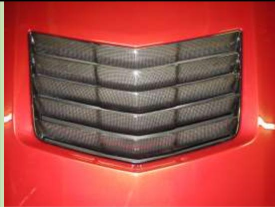
Finished Carbon Fiber Hood Vent in place. Fit is excellent, no gaps and it fits flush like the OEM plastic vent
