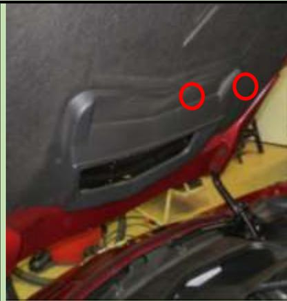
The plastic cover is held on to the plastic hood vent with 4 metal clips. One is shown in this pic. Simply get your fingers behind a corner and pull it off. Note the metal clips will be removed and reused on the CF vent. They need to be spread than closed so the fit tightly on the CF stands that are similar in shape to those on the plastic vent.
