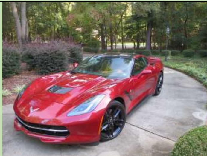
This photo shows the Carbon Fiber OEM roof, the LG Motorsports Carbon Fiber Side Skirts and the Carbon Fiber Hood Vent.
