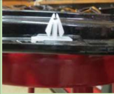
This is the clip removed. Note, just push the clip sideways to remove, it will slip out. May take a bit of force. Be careful, they need to be reused.
