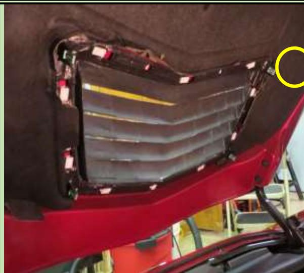
With the 10 clips in place, it's time to press them into the CF vent into the holes in the hood. I used a small screw driver to lift the insulation above the CF hood vent edge. This raised insulation edge will be hidden by the inner plastic cover. I used the side of my closed hand to tap loose clips into the hood.
