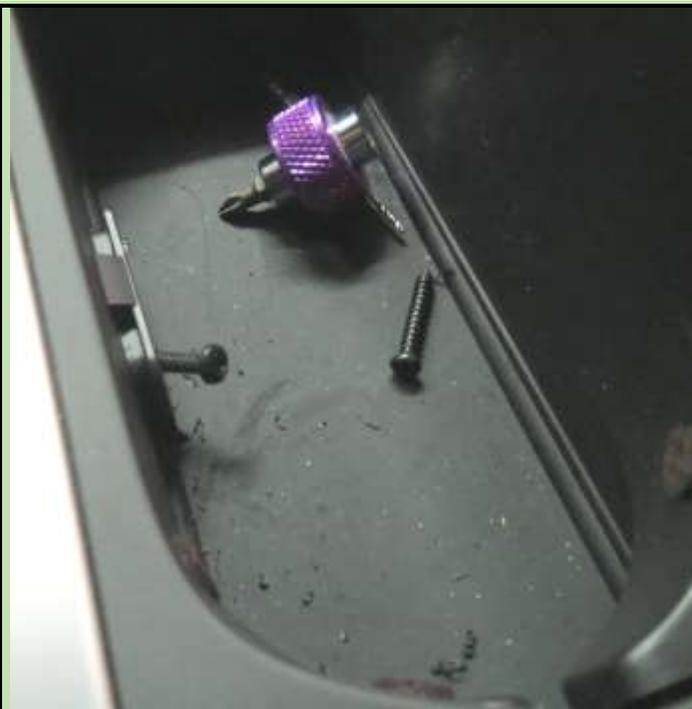
This is a view of a screw inserted into the plastic support to which the *Insert* connects. Unfortunately the unsupported length of the screw allowed the assembly to flex so it was not the ridged one it was hoped would be achieved. All support was also coming from one end of the *Insert*.
