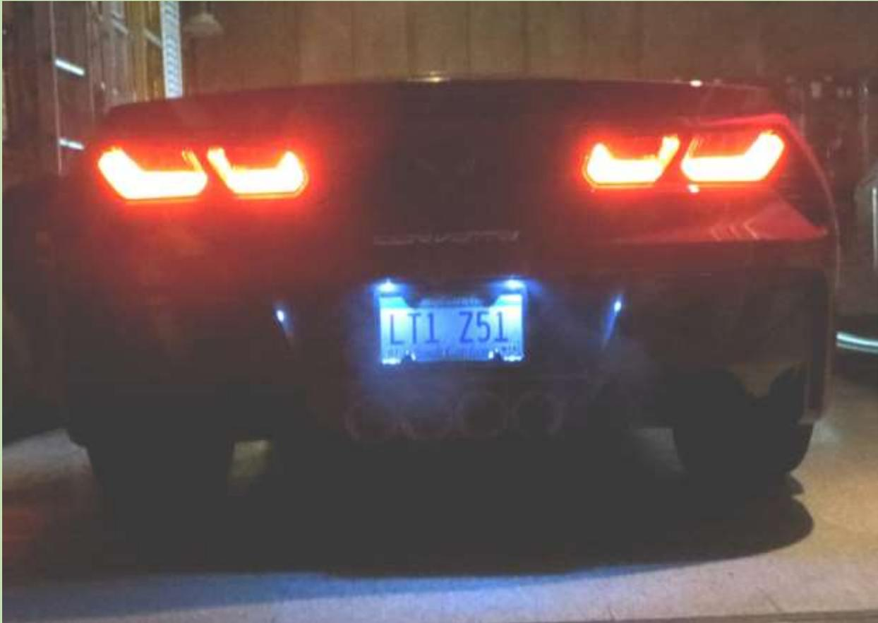
The more visible you can make the Corvette, especially at night, the better! The only bulbs that are not LED's in the C7 are those illuminating the license plate and rear hatch. LED bulbs are available as a replacement. They provide a bright much whiter light.
