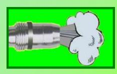
Depending on the number of weld starts, tack welds and how often the MIG wire is just inched to cut of the end or position it in the joint, the gas surge at the weld start can waste over half the shielding gas used!
