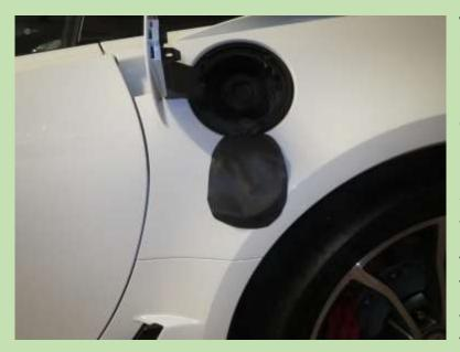
The gas bib for the C7 Corvette attaches to the bottom screw of the ring cover in the fuel door recess. I also placed a washer between the bib and the screw head.
