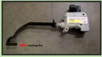
Lock. It is not the mechanical catch that is "push and pop open" but a lock that pushes a "Locking Pin" (see pic left) into a hole in a lid bracket.
