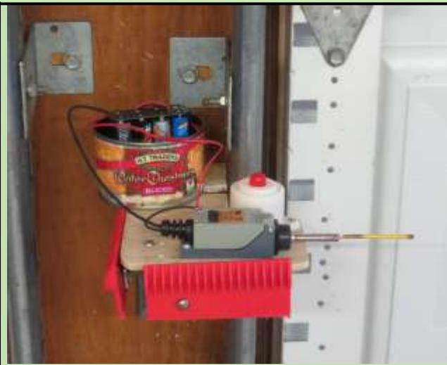
This is the finished assembly with the battery pack in the “vegetable can” holder screwed to the platform! Not quite an Andy Warhol picture but it works. The battery pack can be removed when needed, which hopefully will be seldom.
