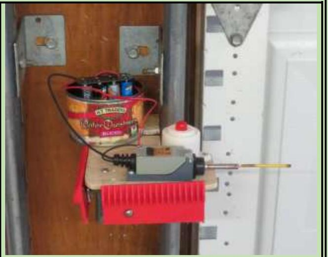
The first step was to build a platform to hold the limit switch, alarm and battery pack. A piece of 1/4 inch plywood was cut to the shape required. A metal "L" bract was attached to the platform and then screwed into the wood panel between the doors.
