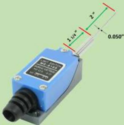
The limit switch selected is a model TZ-8169, a SPDT switch that has a thin, 0.050-inch diameter, 2-inch-long probe wound into a spring that is 1 1/4 inches long before entering the switch. It has both normally closed and normally open terminals. The device only uses the normally open contacts which close if the probe is touched by a mirror.
