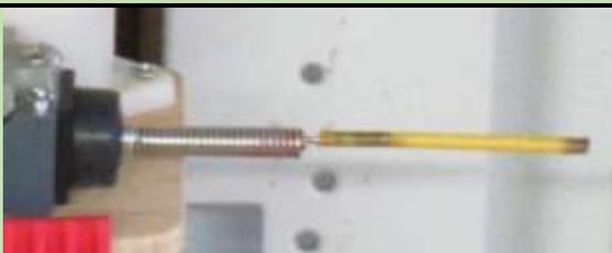
To assure the metal probe does not scratch the mirror, if it ever hits, it was first dipped in liquid plastic. Then a piece of yellow vinyl shrink tubing was placed over the coated wire, extending 1/8 inch past the end. A heat gun secured it to the coated probe.
