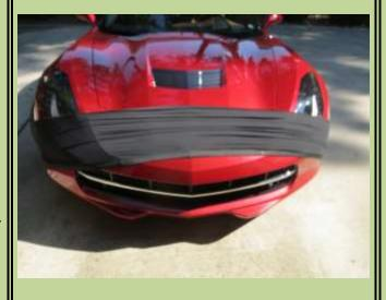
Step 7 may appear confusing until you read the text and then look at this picture. The outside bottom corners will not stay on the edge of the bumper. As noted in the instructions, this next step is optional but recommended. The instructions indicate the bolt that holds the outer edge of the air dam just be loosened to provide a gap for the Bra to fit into. I found it required several turns to provide the needed gap. I was concerned the screw could work loose, especially when not using the Bra..
