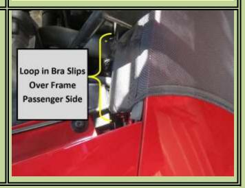
Although not mentioned in the Instructions, I was able to place the "Plastic Cover" back over the Bra loop. It does fit in with friction as noted in the instructions. Note on the passenger side there is a cable that fits over it and helps it stay in place. Since I will only be using the Bra for long trips I might leave them off until I remove the Bra
