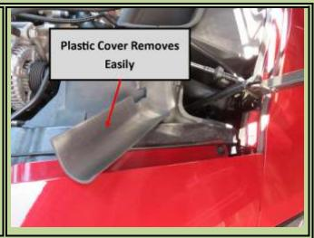
This is the driver's side with the "Plastic Cover" removed and the referenced "Frame" (noted in the instructions) exposed. That "Frame" is where you'll attach the loops that are on the ends of the Bra.
