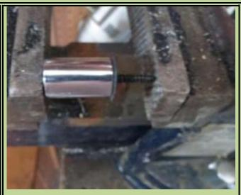
The washer will deform slightly but one blow from a hammer on the vise anvil quickly flattened it. It slipped over the supplied snap without having to ream out the hole.
