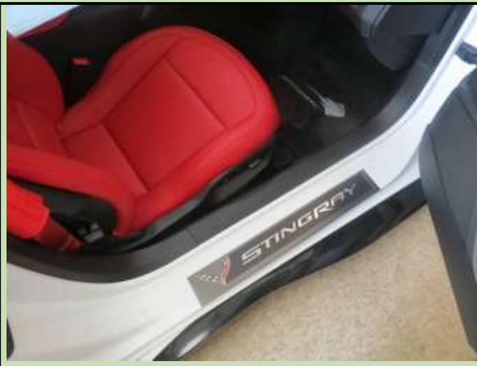
The 7 clips were easily located in the slots. Once in they were in place, the Stingray sill plate was “punched-in” with the side of my closed fist. The clips all snapped in easily. This picture shows it installed.
