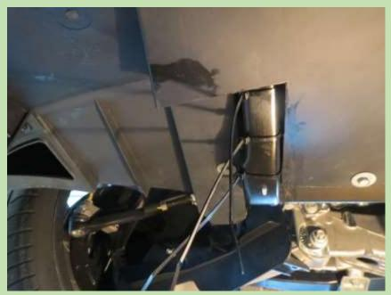
The Grand Sport and my prior 2014 C7 Corvette similar to predecessors: there is not a lot of ground clearance! The first item to scrap when leaving a driveway, etc. or going over a very high, speed bump is the air dam. The flexible air dam is designed to makes a scrap and modest noise. However not much higher and the next item to scrap is what GM calls
