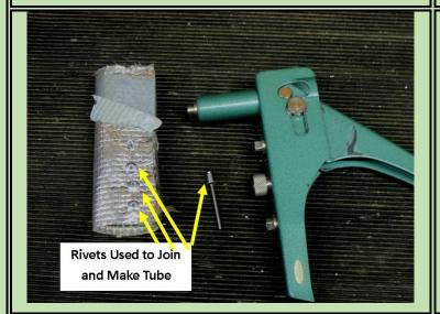
Cut the material and unlike the high temp sealer/glue I used when installing on parts of the street rod (since I did not have any left) decided my seldom used rivet gun would work fine. Used an awl to punch holes into the folded material and the rivet gun make quick work of installing the rivets. Held the shape in place with duct tape that was peeled back as the string of rivets was put in along the seam.
