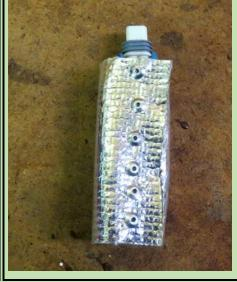
Hard to see the insulated tube over the solenoid connector since it is up rather high on the transmission left side. However the same type of insulation is installed over the temperature sensor that is located near the bottom. The lower one is close to the exhaust pipe and is no doubt why it is used. The wires also have an insulation covering.
