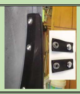
The 1 inch long snap screws (shown installed left) are needed to reach through the winglet supports held the winglet fine. The original screws were shorter as noted in the above pic (black screws with washers.)
