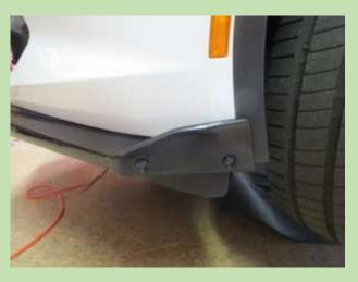
The Stage 3 Winglets also have a major function for me. It helps integrate the "spats" that the Grand Sport (and Z06) use to handle the wider front tires (285 versus 245 in the base and Z51.) Thought the "spats" looked like a cheap add-on! OK for my V8 powered 1974 Jeep Renegade! Could justify that approach for the rag top Jeep but for a Corvette?
