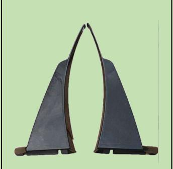
The Stage 2 winglets are held in place with 6 mm visible bolts that are screwed into threads formed in the carbon flash painted, carbon fiber splitter.
