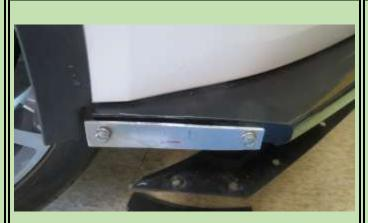
The flat plastic splitter bottom screws were removed to check clearance and since they will be replaced with "Splitter Guards" (more on those at the end!)
