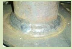
and was weld getting start porosity on most parts. He had adjusted all welding parameters including gas flow rate
