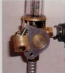
The company installed flow-rate limiters that cap the flow of weld gases so that welding specifications cannot be exceeded.
