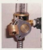
has improved weld quality while simultaneously reducing weld costs by installing flow rate limiters on each of their company's 30 MIG welding stations.
