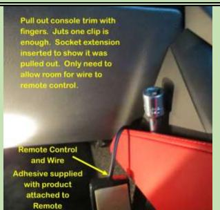
The next step takes a little more force. The console trim, like others used on the C7, is held with strong clips. However, they are very rugged and are easily put back once unclipped, just by pressing.
