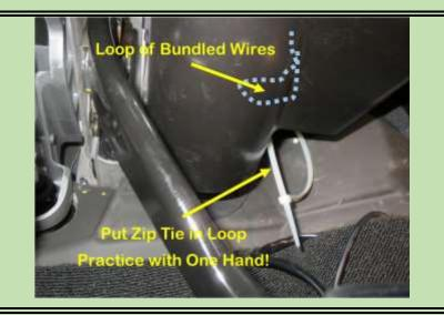
Tried slipping the Controller though the Zip Tie and tightening around the wires. NO GOOD! Pulled out one of the connectors from the Controller! Started the car and check engine light came on!
