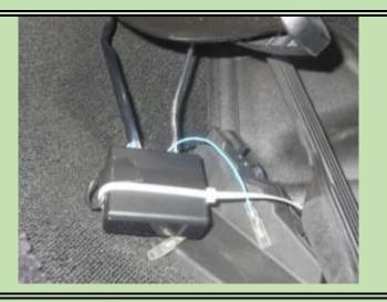
A Zip Tie was put through the "O" Ring and the Controller body. It was pulled tight and the tail subsequently clipped.
