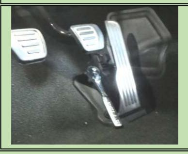
Use a 10 mm socket and remove the bolt. The Pedal has clips on the bottom side toward the seat that slip into recesses in the floor. Don't pull up on the Pedal assembly. First pull back toward the seat with it pressed in the floor. It's like pulling your foot out of slippers with an open back!
