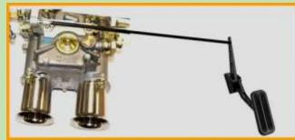
Remember when all there was between the gas pedal and the air/fuel induction system was a simple cable or rod? Be it a carburetor or air control throttle body it was just a mechanical link. *No more!* Today, like most other things in your car the link is controlled by a
