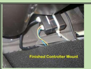
This is the finished mount. The Controller is held securely to a wire bundle under the dash. A strong "O" Ring is secured to the Controller with "Stick Ass Tape" to assure it does not slide and a Zip Tie that will be more than strong enough to hold the light weight Controller.
