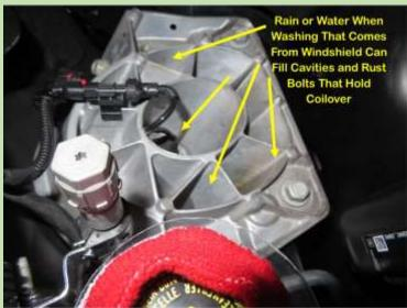
has rusted the coilover bolts. Some have removed 6 or more ounces of water from the deep cavities.
