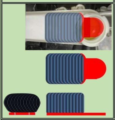
From Forum Member observations and one using a remote fiber optic camera video of Fluid Leaving and Returning it appears the fluid Max level is much higher than needed. He lowered his to a ¼ of the bottom reservoir. Works fine. Forum members have shown, so far, that they have no leaking with a lowered fluid level and the Lift works fine.
