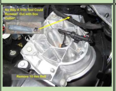
First step on the Driver's Side is to remove the clamp holding a wire bundle. It says use a "forked" Trim Tool. As noted above I have 3 different "forked" ends with different bends. Would not budge! Tried a large screwdriver and it moved a bit, but no way was it coming out!
