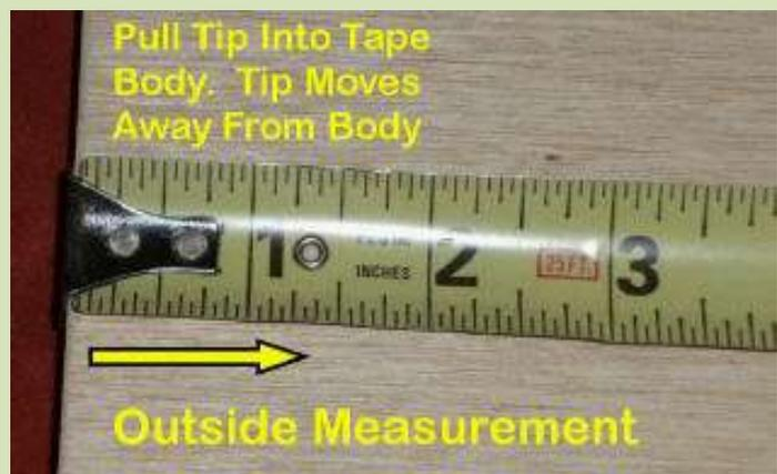
The tape is pulled slightly away from the edge being measured and the tab moves slightly to the left in this case. It moves the thickness of the tab so that the zero point is now on the inside or from the photo the right side of the tab. This places the zero location as necessary to have it measure properly.
