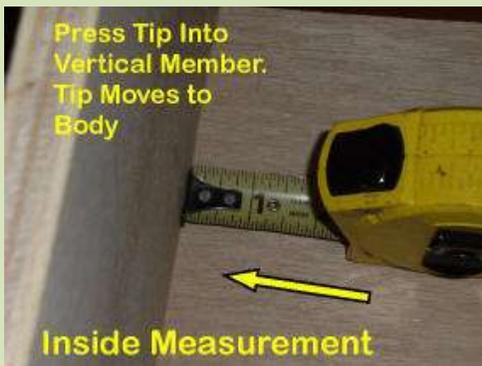
As seen in the picture above there is a metal tab at the start end of the tape. It is usually attached with two rivets. However it is loose. **Do Not** tighten these rivets with a hammer! The tab is loose for a reason.
