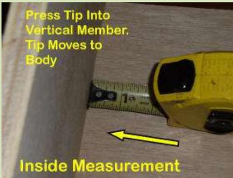
As seen in the picture above there is a metal tab at the start end of the tape. It is usually attached with two rivets. However it is loose. **Do Not** tighten these rivets with a hammer! The tab is loose for a reason.
