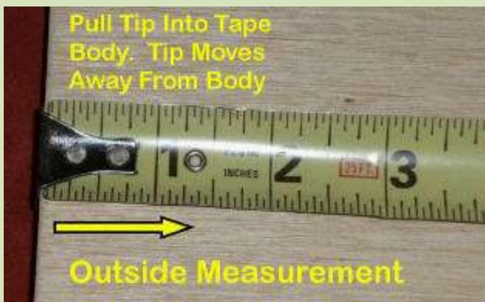
The tape is pulled slightly away from the edge being measured and the tab moves slightly to the left in this case. It moves the thickness of the tab so that the zero point is now on the inside or from the photo the right side of the tab. This places the zero location as necessary to have it measure properly.
