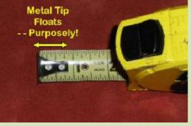
As seen in the picture above there is a metal tab at the start end of the tape. It is usually attached with two rivets. However it is loose. **Do Not** tighten these rivets with a hammer! The tab is loose for a reason.
