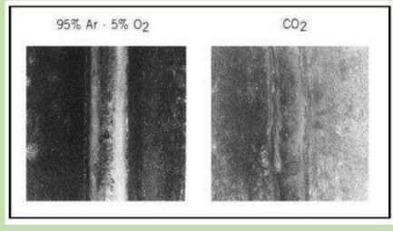
However, as mentioned CO<sub>2</sub> will not produce spray transfer but can be used for Short Arc welding. The maior drawback of using pure CO<sub>2</sub> is the harsh globular metal transfer causes hiah weld spatter levels. The weld surface resulting from pure shielding is also more heavily oxidized than
