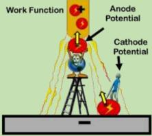
How the arc attaches to the wire tip and drop also has a major affect on the overall arc stability and spatter generation. When MIG was first introduced
