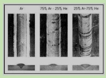
Argon-Helium: These mixtures are used for welding aluminum, copper, and nickel alloys. These qases are used in various combinations and increase the voltage and heat of MIG as more Helium is added. To maintain better stability characteristics arc а minimum of 20% Argon is needed. Generally, the heavier the material the higher the percentage of Helium. Mixtures typically range from 20 to 75% Helium. The figure left shows weld beads made with several Argon
