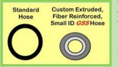
We have invented and patented a system to reduce this "gas blast" by about 85% while maintaining the system pressure and enough extra gas to purge the weld start area of air. It's called the *Gas Saver System* ( $GSS^{TM}$ .) It consists of a small ID, very heavy wall, custom extruded gas delivery hose that holds much less gas when welding stops and doesn't expand when the pressure increases.
