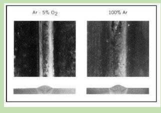
TIG welding was developed on the early 1940's before MIG. Pure Helium or Argon was needed for that process to not only protect the weld but also the tungsten electrode. Even small amounts of Oxygen will contaminate the tungsten electrode in a short time. For MIG, pure Argon or Helium and Argon/Helium mixtures worked well for welding aluminum but when welding steel it was found that to obtain a quality arc and smooth metal transfer,
