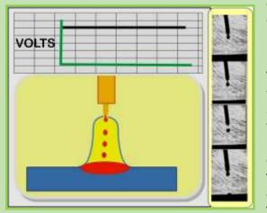
This mode of metal transfer is hot and would make welding out of position very difficult or require very small ID wires. In fact some wires as small as 0.020 inch OD were employed. Tough to feed!
